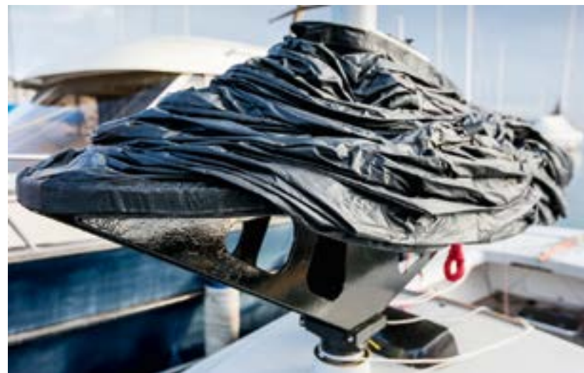
Sailcloth is inexpensive basic parachute material which folds down to minimal size and requires only light pressure to keep inflated. Reefing simply requires lowering the mast and hauling on a reefing line
