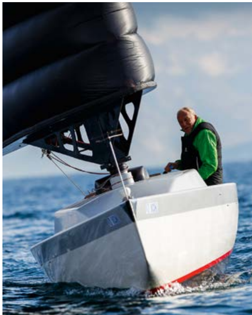
Edouard Kessi and business partner Laurent de Kalbermatten created the Inflated Wing Sail (IWS) and have proved its versatility on a 5.5m hull
