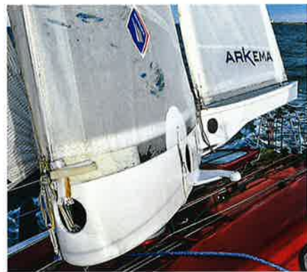
Above: a close-up view of the two-element soft rig on Arkema 3 . The top and bottom rigid control components of these soft rigs are what is attracting particularly keen interest from America's Cup teams designing twin-skin AC75 rigs for 2021. The VPLP soft wing programme ( left ) has the widest scope of the current research projects being focused as it is on both the leisure sailing market (where VPLP is now allied with a 'large manufacturer') as well as on the commercial shipping sector in the seemingly endless quest to find an efficient but also workable wind-powered solution to reducing fossil fuel use at sea
