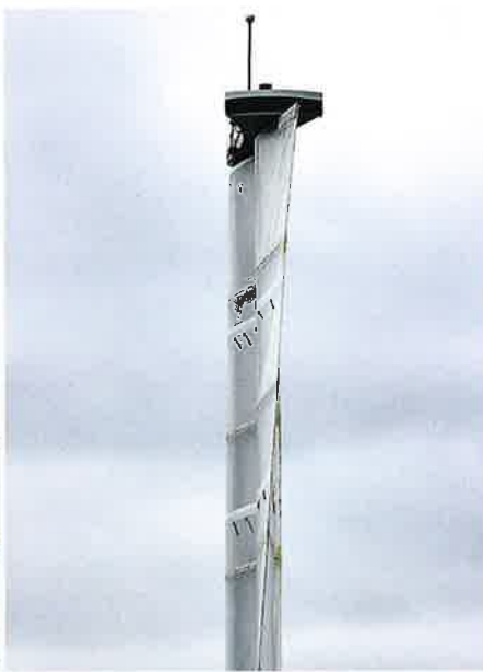
Above: a close-up view of the two-element soft rig on Arkema 3 . The top and bottom rigid control components of these soft rigs are what is attracting particularly keen interest from America's Cup teams designing twin-skin AC75 rigs for 2021. The VPLP soft wing programme ( left ) has the widest scope of the current research projects being focused as it is on both the leisure sailing market (where VPLP is now allied with a 'large manufacturer') as well as on the commercial shipping sector in the seemingly endless quest to find an efficient but also workable wind-powered solution to reducing fossil fuel use at sea
