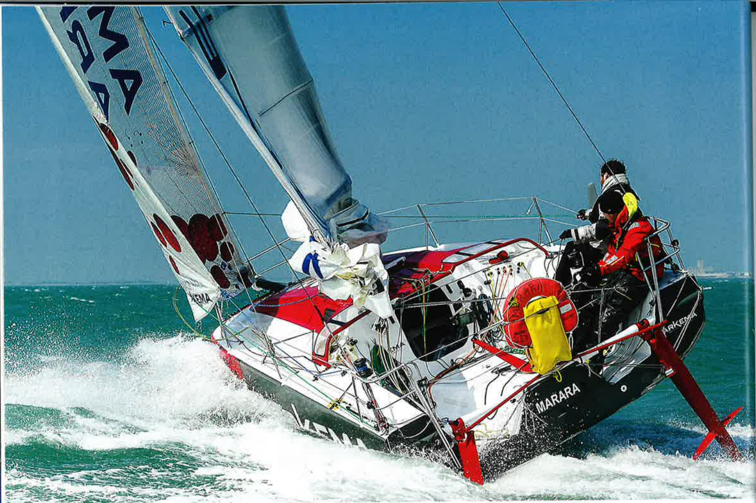
Led by engineer and designer Romaric Neyhousser, the Arkema Mini project is the most ambitious of the current initiatives as it attempts to tackle several new technologies simultaneously. A foiling scow with a fore-and-aft, two-element soft wing rig is a lot to deal with, but Arkema has performed well on the Mini circuit since launching last year. Neyhousser works closely with Guillaume Verdier on his foil engineering and was a member of Verdier's team working alongside America's Cup winners Team New Zealand
